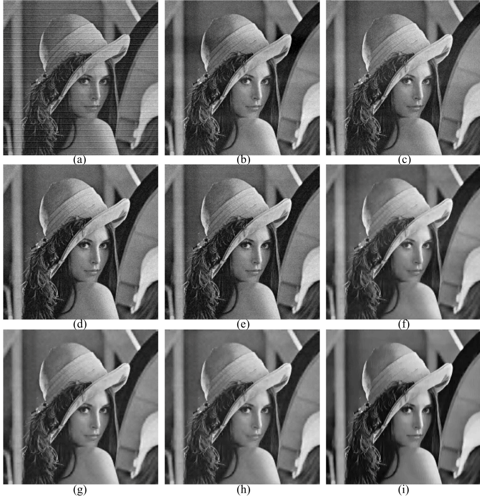
Fig. 5. Simulated experiment using image with random noise. (a) Striped image with Gaussian noise. Destriping results obtained using (b) wavelet-FFT, (c) Uni-TV, (d) VSNR, (e) proposed model without framelet regularization (FR) term, (f) Uni-TV + wavelet shrinkage (WS), (g) VSNR + WS, (h) proposed model without framelet regularization (FR) term + WS, and (i) complete proposed method.
