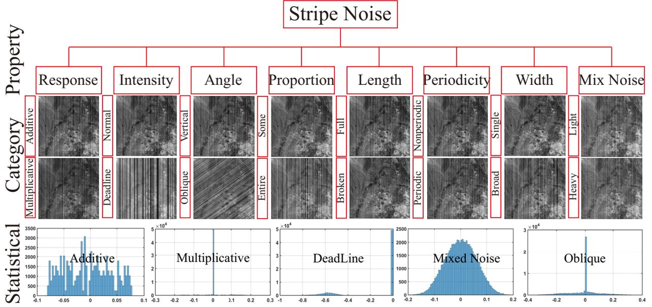
Figure 1. The category of the stripe noise. We classify the stripe noise in both the push-broom (representative hyperspectral imaging) and cross-track (representative MODIS) from their appearances into sixteen classes. Their visual images are shown in the second row. Some statistical histograms of the representative stripes are shown in the last row, which is very different for each stripe.
