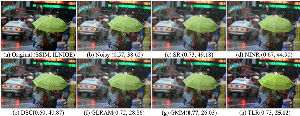
Figure 5. Simulated rain streak removal results of the dataset [19]. The rain streak here is light but dense.
