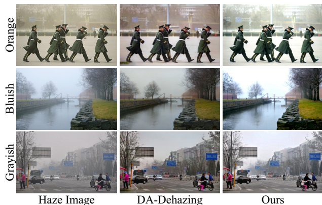
Figure 1. The visual examples of dehazing results for real-world varicolored haze images. The second and third column show the results of DA-Dehazing [42] and proposed method, respectively.
