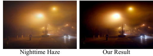
Figure 9. Analysis of the limitation of the proposed PDI2A. Left: real-world nighttime haze images. Right: results produced by PDI2A. Due to huge difference between daytime and nighttime haze images, our method could remove most haze effects while leaving the halo effect behind.
