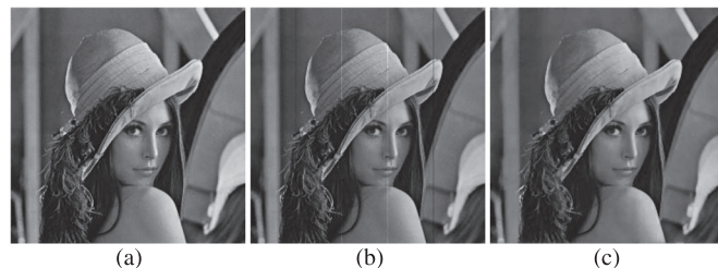
Fig. 22. Simulated destriping result for multiplicative stripe. (a) Original image Lena. (b) Degrade by multiplicative stripe. (c) Our LRSID result.
