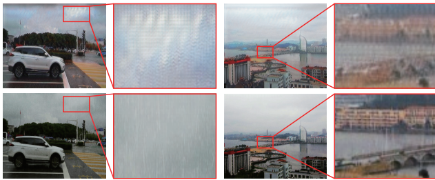
Figure 9. The superiority of translation between rain layers. Top: CycleGAN directly translates background into rainy image leaving obvious artifact. Bottom: JRGR preserves the background and focuses on the translation of rain layer, obtaining natural result.
